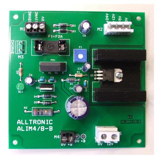
CAUTION: Before connecting the 230V check the correct connection of the wires 0V and +12 V (sensors) because, if reversed, causing the burning of all the ICs of the control.
